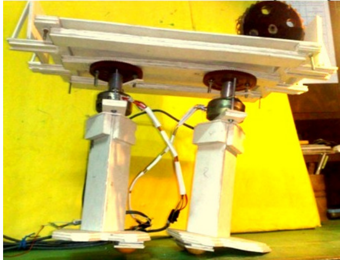
Figure.9. Slant position due to displacement of the moving mass
