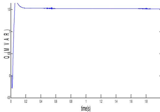
Fig 5 Reactive power output of Wind farm
