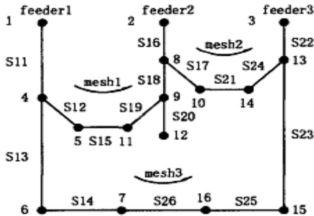
Fig. 3 Single line diagram of three feeder system
