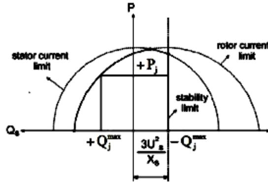
Fig.2. DFIG capability limits curve
