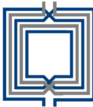
Figure 2.4.3: Segmented and Interleaved stacked transformer (two plane).
