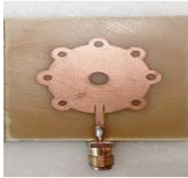
Figure 6. Fabricated prototype of proposed circular fractal antenna Table 3: Comparison of designed antenna with existing antennas
