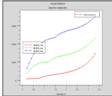
Figure 6 : SELBOX structure ID-VDS graph for 0.001 micron gap length At V = 1v, 2v, 3v
