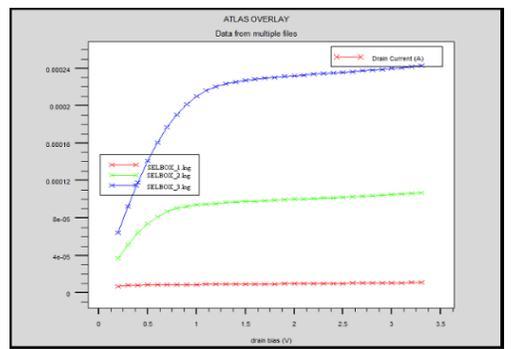
Figure 12: SELBOX structure ID-VDS graph for 0.2 micron gap length At VG = 1v, 2v, 3v
