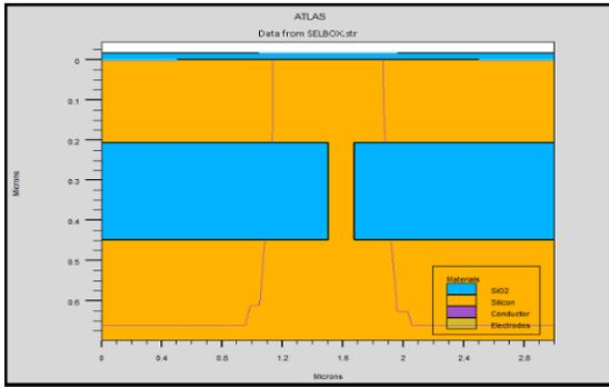
Figure 11: SELBOX structure with gap length 0.2 micron
