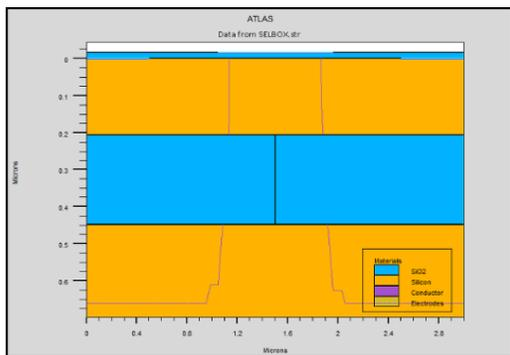
Figure 7: SELBOX structure with gap length 0.01micron
