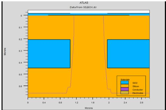
Figure 12: SELBOX structure with gap length 1micron
