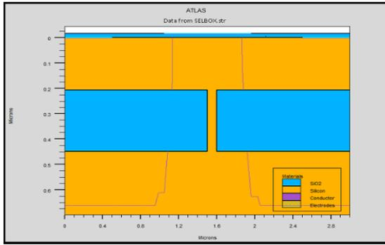
figure 9: selbox structure with gap length 0.1micron
