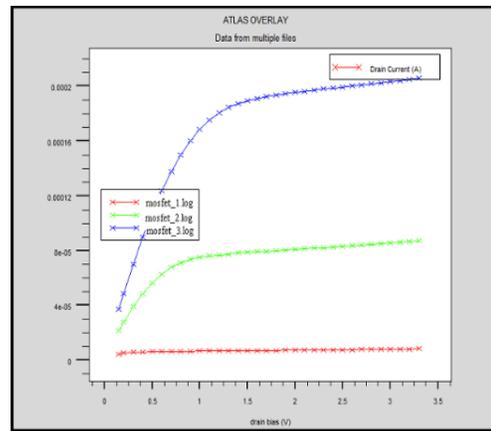
Figure 2: MOSFET ID – VDS for ramp gate voltage (VG) 1v, 2v & 3v
