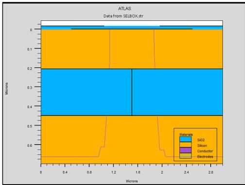
Figure 5 : SELBOX structure with gap length 0.001micron
