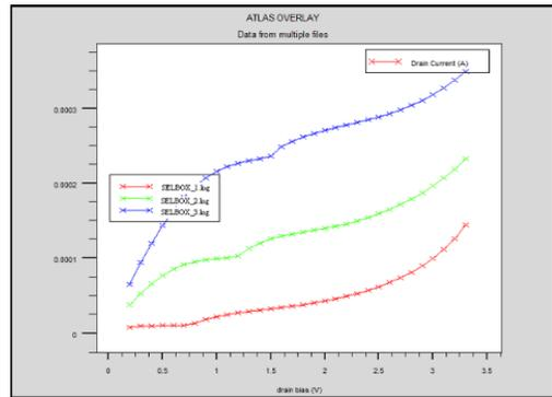
Figure 8: SELBOX structure ID-VDS graph for 0.01-micron gap length At VG = 1v, 2v, 3v
