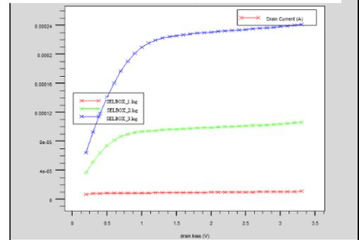
Figure 13: SELBOX structure ID-VDS graph for 1 micron gap length At VG = 1v, 2v, 3v
