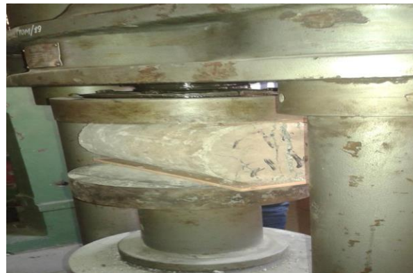
Figure No.9. Split tensile Test on Geopolymer concrete
