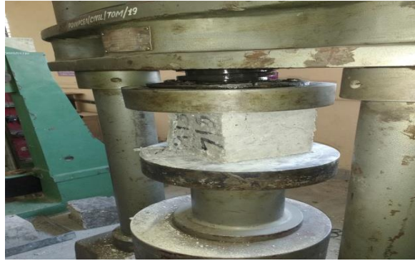
Figure No. 1. Compressive tests on Geopolymer concrete
