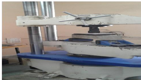
Figure No.7. Flexure test on geopolymer concrete
