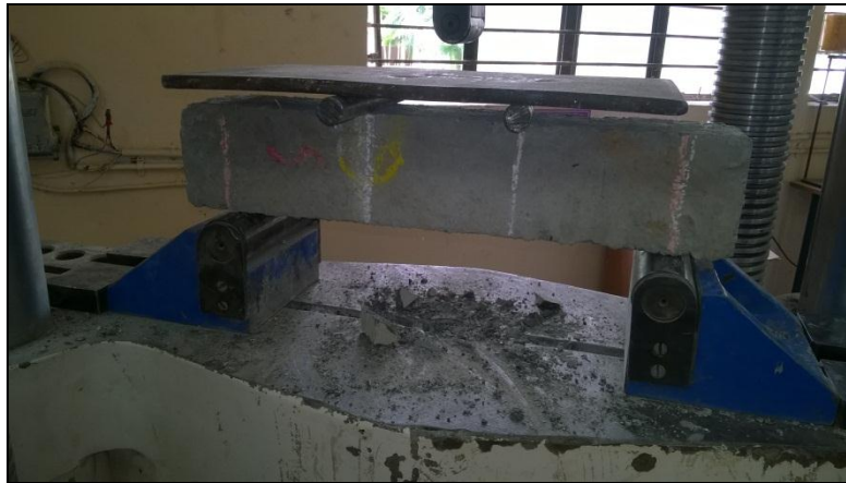
Figure 5- Flexural Strength Test Setup
