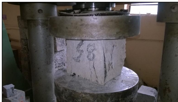
Figure 3- Compressive Strength Test Setup
