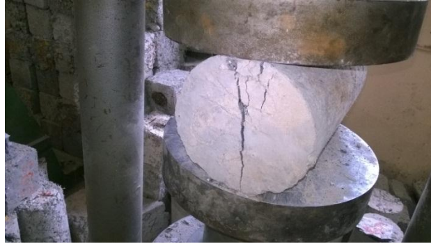
Figure 4 - Spilt Tensile Strength Test Setup
